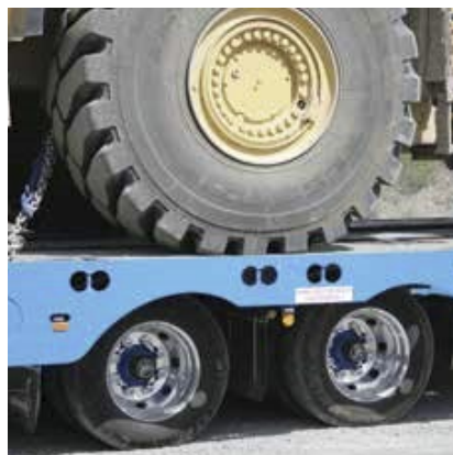
Above left: Loading a Container on the Drake built low loader on BPW 8 stud 275PCD 19.5" drum brake fixed axles with OT heavy duty underslung suspension. (Supplied by Southern Cross heavy Haulage)
