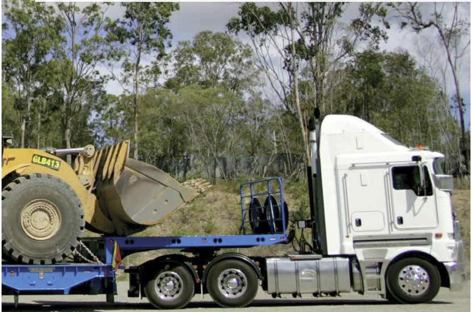
The 14 metre Drake quad-axle drop deck low loader ready to cart a 980 CAT loader from Southern Cross Heavy Haulage depot - Stapleton, Queensland to Western Australia.
