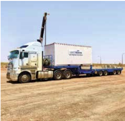
Above left: Loading a Container on the Drake built low loader on BPW 8 stud 275PCD 19.5" drum brake fixed axles with OT heavy duty underslung suspension. (Supplied by Southern Cross heavy Haulage)
